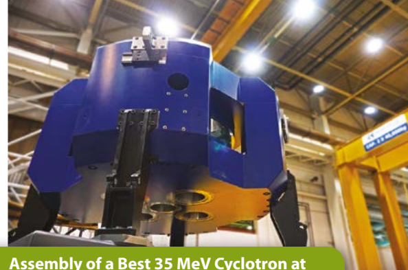
Assembly of a Best 35 MeV Cyclotron at Best Theratronics facility, Ottawa, Ontario, CA
