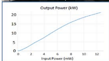
3 x 8kW amplifiers combined
