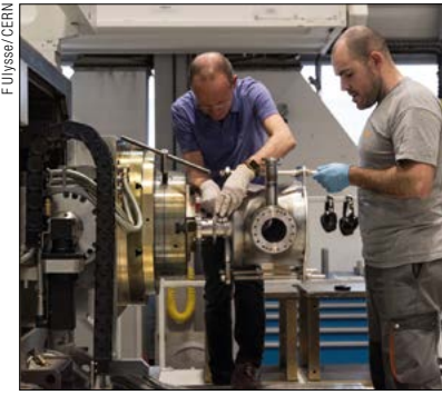
First niobium crab cavity fabricated at CERN for the High-Luminosity LHC project.
